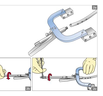
Now a nail of appropriate length and diameter is connected with the targeting device. The cambered, bevelled, proximal end of nail fits in the fish-jaw-type groove of the adapter. Afterwards, the adapter screw is tightened with the tightening sleeve using the socked key. Only in this case targeting accuracy for proximal interlocking can be enabled.
