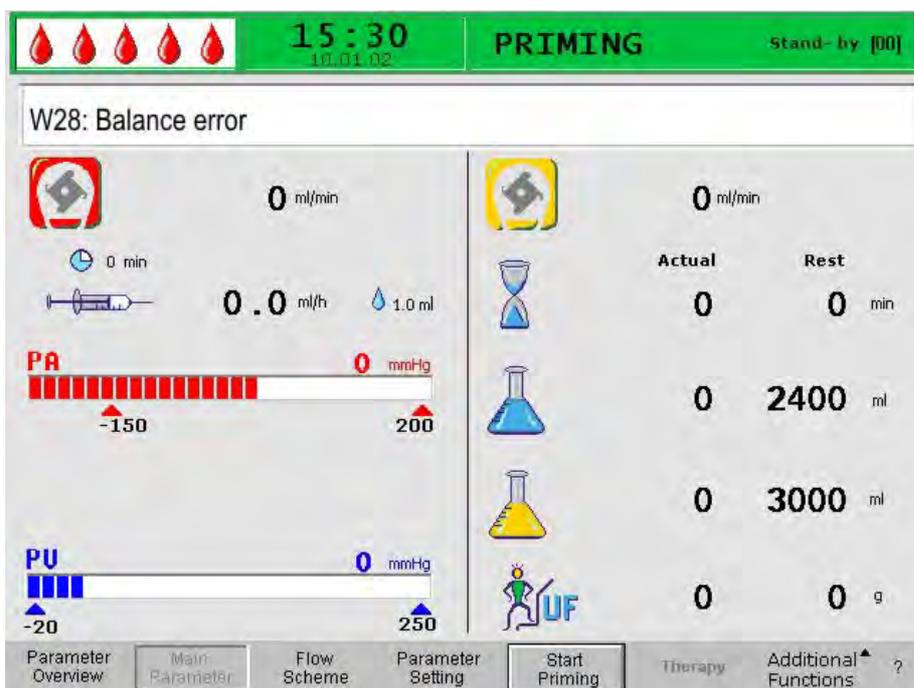
Fig. 10-3 Warning message in the Alarm/Note line
