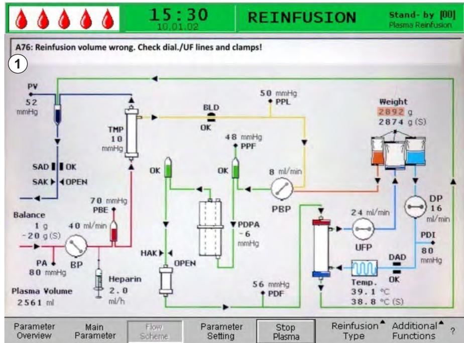
Fig. 10-1 Alarm indication in Alarm/Note line
