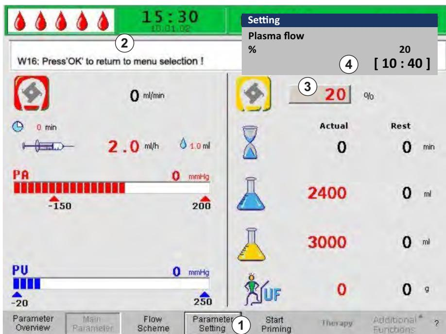
Fig. 3-18 Parameter selection in the *Main Parameter* screen
