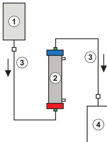
Fig. 10-11 Set-up for ultrafilter rinsing
