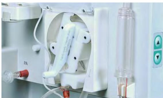
Fig. 10-12 Crank on blood pump
