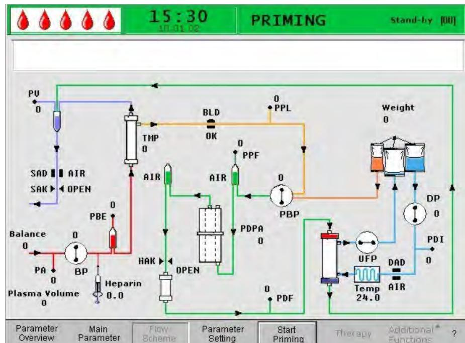
Fig. 6-5 Flow Scheme screen in the priming phase
