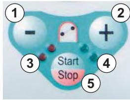
Fig. 3-9 Blood pump operating keys
