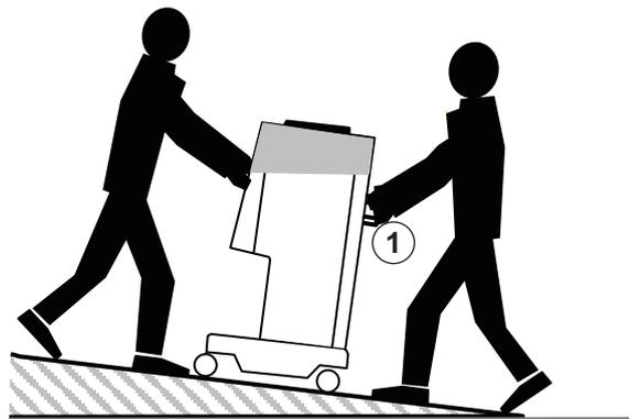
Fig. 4-1 Moving the machine on stairs and slopes (2 persons)
