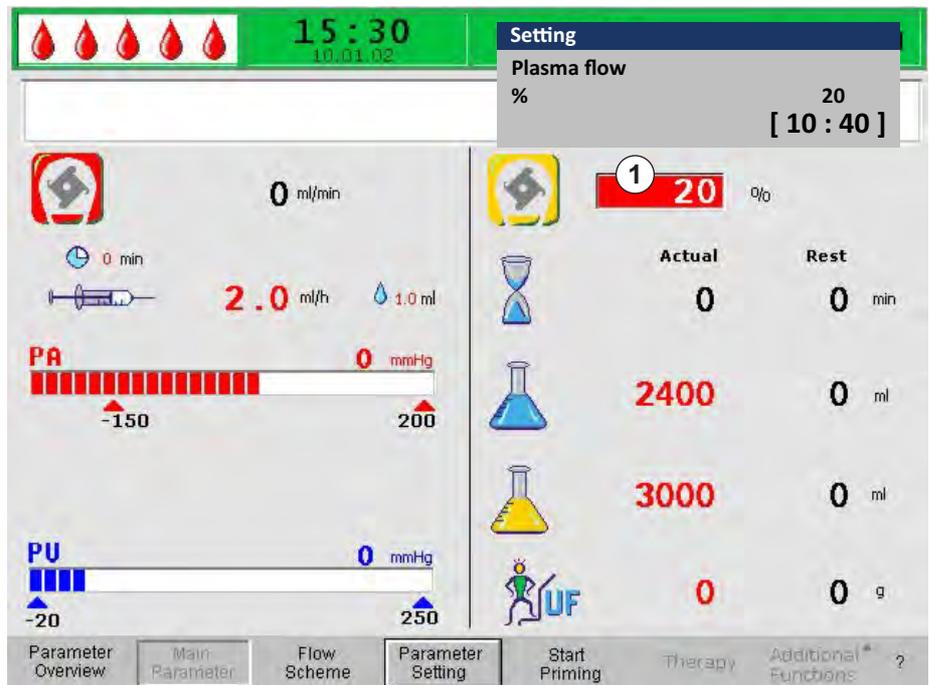
Fig. 3-19 Parameter setting in the *Main Parameter* screen
