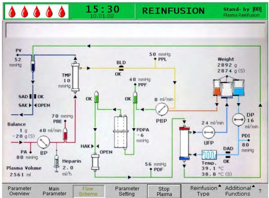
Fig. 8-10 Flow Scheme screen in the reinfusion phase
