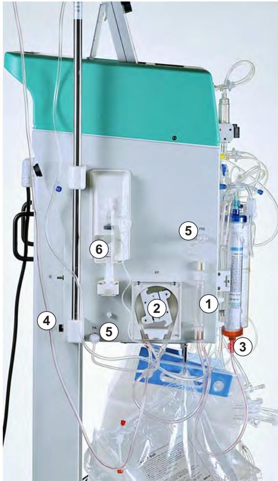
Fig. 5-13 Setting-up the arterial line
