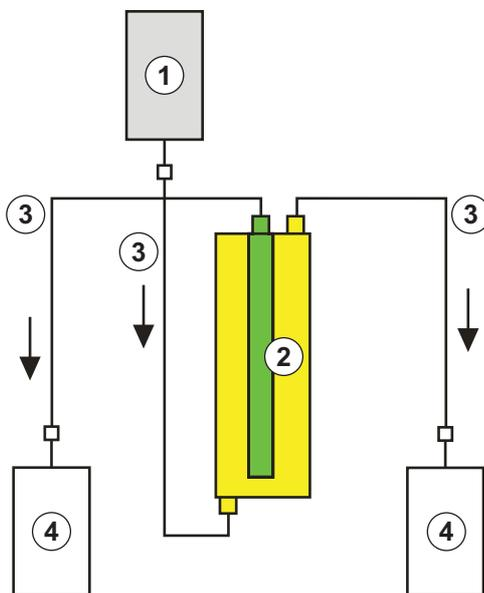
Fig. 10-9 Set-up for precipitate filter rinsing
