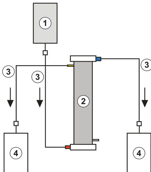
Fig. 10-8 Set-up for plasma filter rinsing
