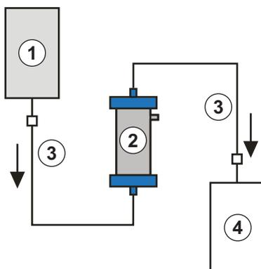
Fig. 10-10 Set-up for heparin adsorber rinsing
